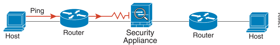
Figure 37-5 Ping Failure Because the ASA is Not Translating Addresses
