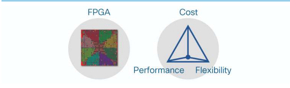
DIAGRAM FPGA - More Cost, Moderate Flexibility, Moderate Performance
