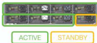
DIAGRAM N+1 Power Redundancy Mode
