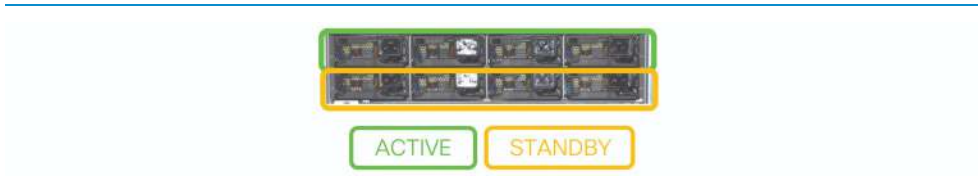
DIAGRAM N+N Power Redundancy Mode
