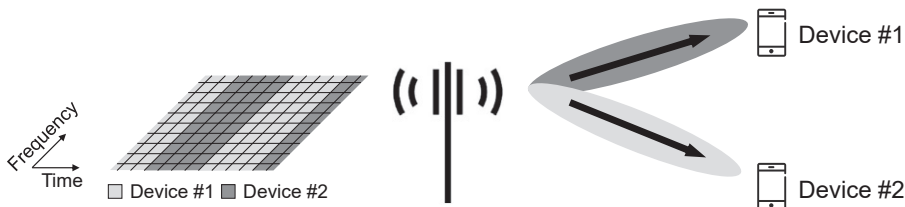
Fig. 11.4 Time-domain (non-simultaneous) beam-forming in multiple directions.
