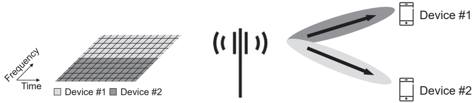
Fig. 11.5 Simultaneous (frequency-multiplexed) beam-forming in multiple directions.
