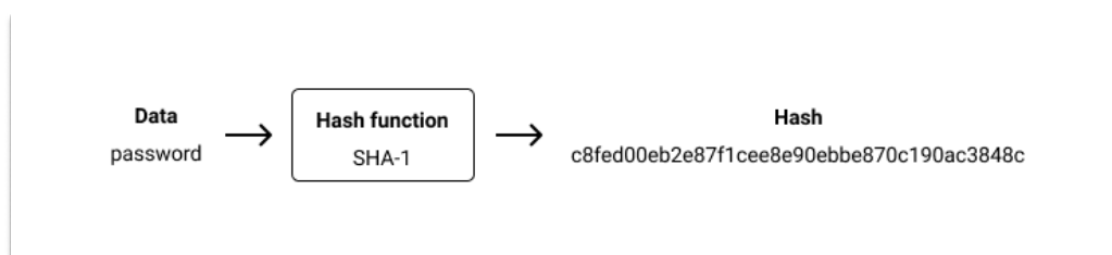
Figure 5.4: How a hashing function works
