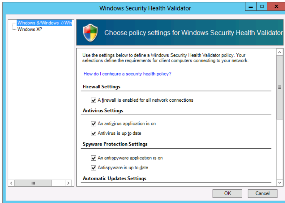
FIGURE 7-7 Specifying settings for a new SHV configuration
