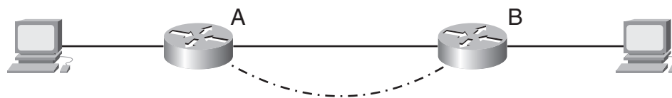
Figure 1-6 Increasing Redundancy to Increase Network Resilience
