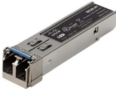
FIGURE 7.2 SFP+ for fiberoptic Ethernet
