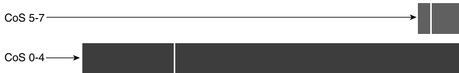
Figure 10-6 Basic Catalyst Queuing: 2Q2T Example—CoS-to-Queue Mappings
