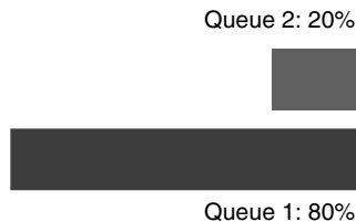
Figure 10-4 Basic Catalyst Queuing: 2Q2T Example—Buffer Allocation
