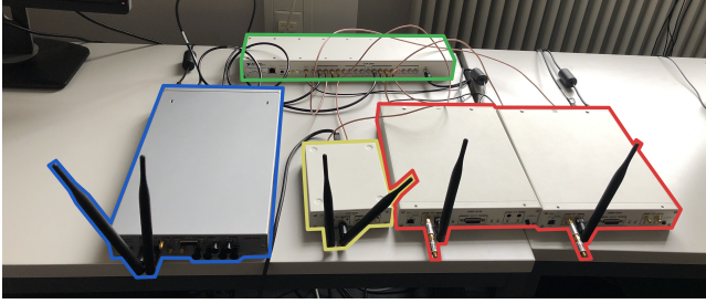
Figure 9: Our setup used for the evaluation of the passive localization and the IMSI Extractor.
