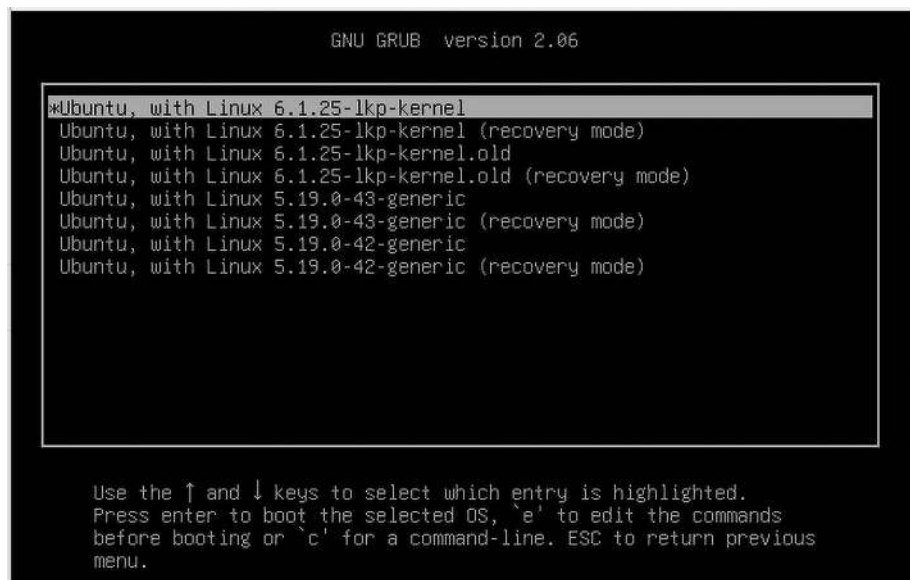
Figure 3.5: The GRUB2 Advanced options... menu showing available kernels to boot from
