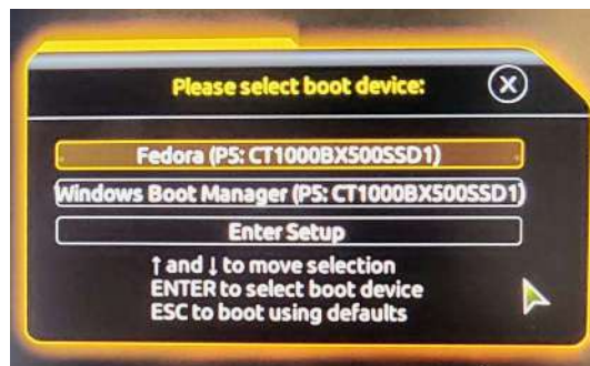
Figure 3.6: The boot selection menu on a UEFI-based x86_64 PC
