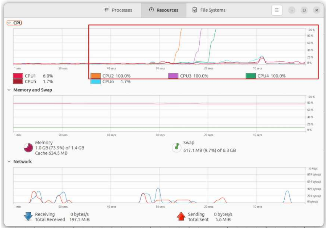
Figure 10.4: Screenshot showing the gnome-system-monitor GUI app; our three “ yes ” processes can be seen hammering away at 100% CPU usage on their three designated CPU cores (CPU2, CPU3, and CPU4)
