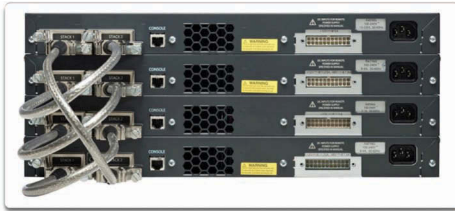
Figure 3-49 Cisco Catalyst 3750 Switch Stack
