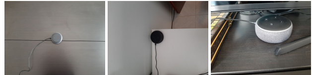
Figure 5: Placement of the Echo Device in the Open (left), Wall (center) and Small (right) Scenarios.
