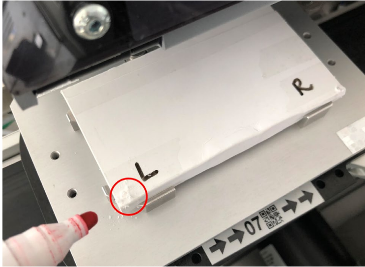
Figure 32. Data mangling on the MES, Step 5: The drill unexpectedly drills on the left.
