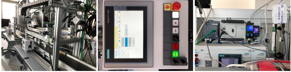
Figure 4. Details of a machine (drill), HMI, and PLC in the target manufacturing system
