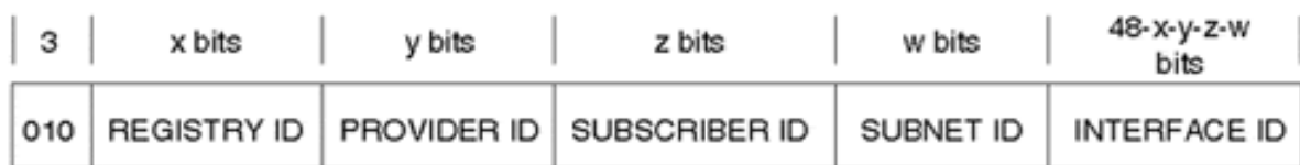
Figure 3-22. IPv6: Provider-Based Unicast Address Format
