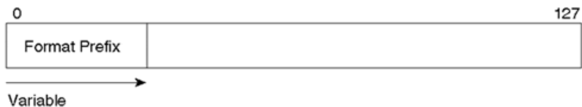
Figure 3-21. IPv6 Prefix and Address Format
