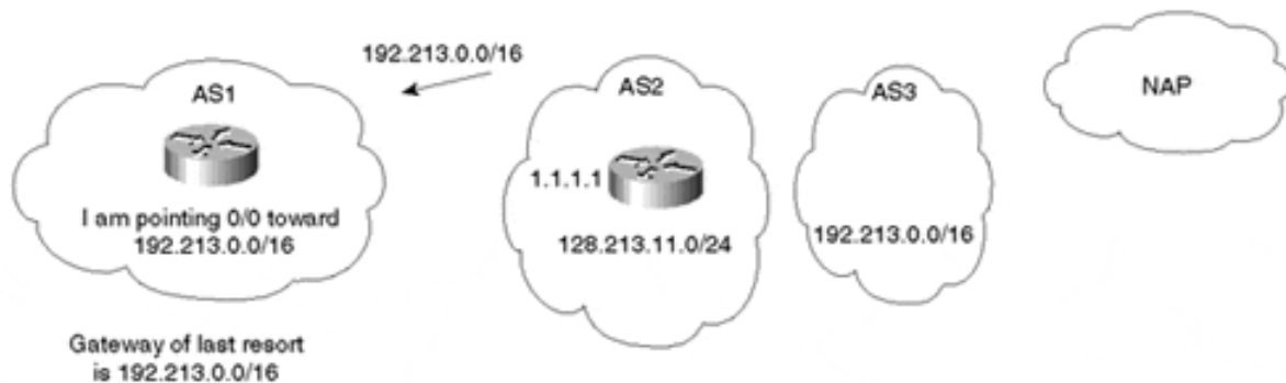
Figure 7-4. Pointing Default Toward a Network Number
