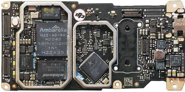
Figure 4. Main board shows the Atheros AR1021X-CL3D Wi-Fi module located in the middle of the board
