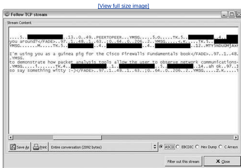
Figure A-2. Displaying a TCP Communications Stream
