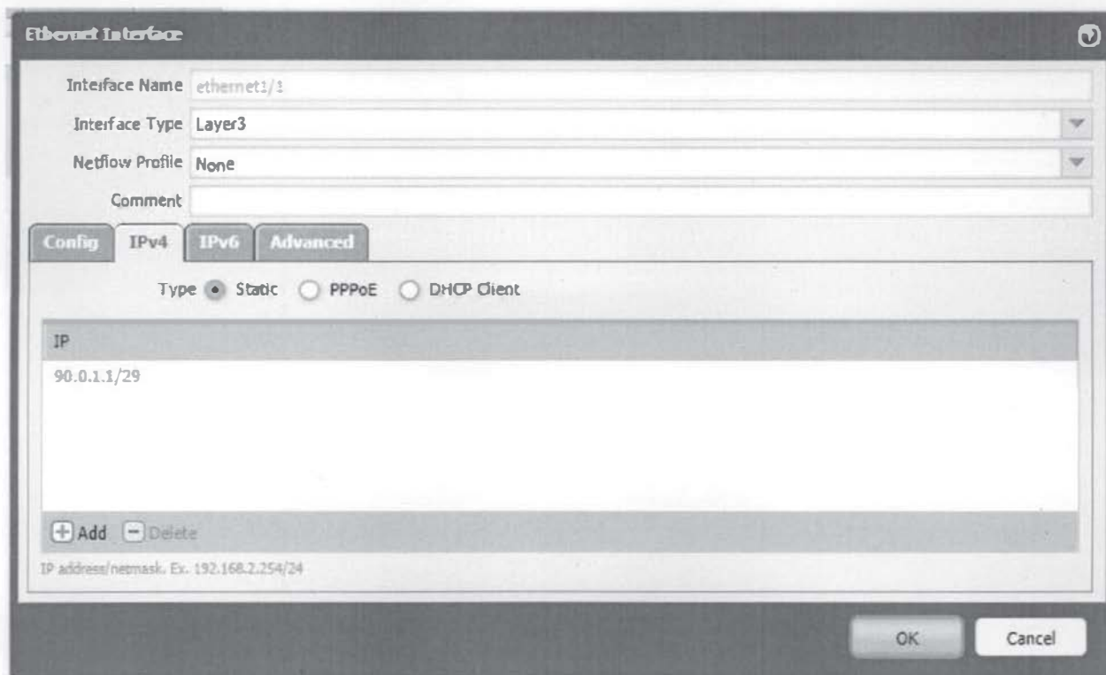
Figure 3. 5 IP address configuration on the interface
