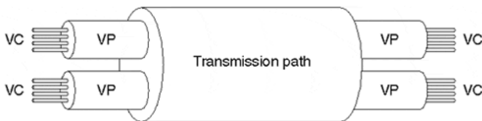
Figure 8-3 Bundling of Multiple VCs in a VP
