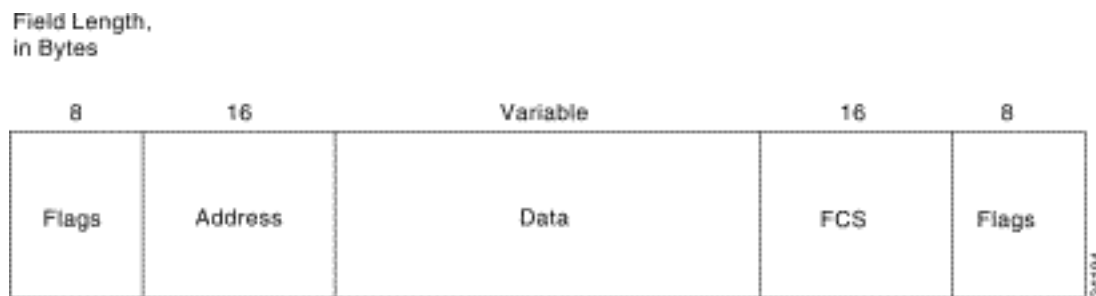
Figure 10-4: Five fields comprise the Frame Relay frame.
