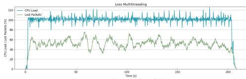
Fig. 6: KeyTrap attack on Unbound with 1 request and 2 threads.
