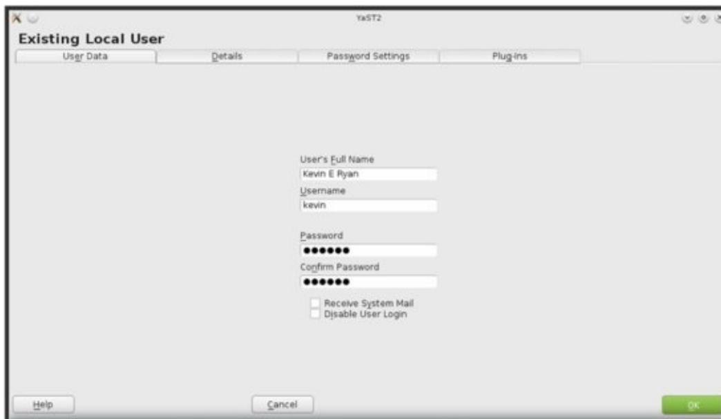
Figure 13.3 The Existing Local User dialog box enables you to edit a wide variety of account properties.
