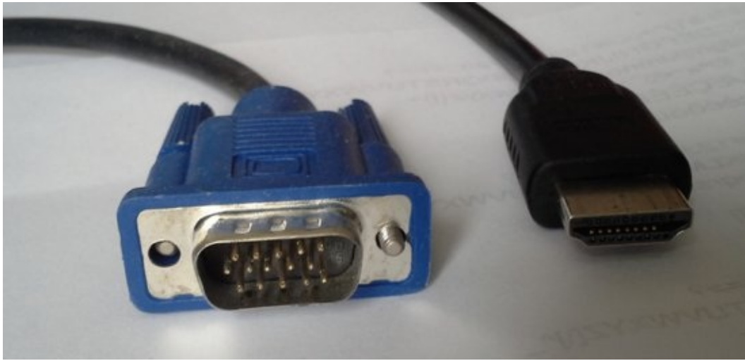
Figure 5.4 VGA connectors (left) were common in years past and are still available today; HDMI connectors (right) are common on newer monitors and video cards.
