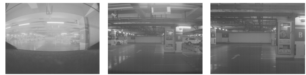
Figure 15: Three kinds of camera images dumped from GPU memory. Left one is the fisheye image; middle one is the main image and right one is the narrow image. We found that the lane detection is based on the main image.
