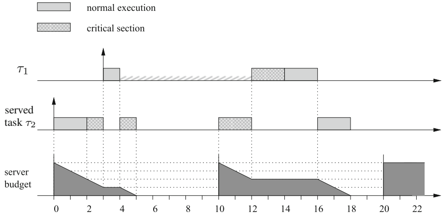
Fig. 9.21 Example of extra blocking introduced when the budget is exhausted inside a critical section
