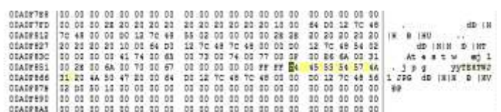
Figure 2 The data remnants of GDA-Upload by FTK Imager
