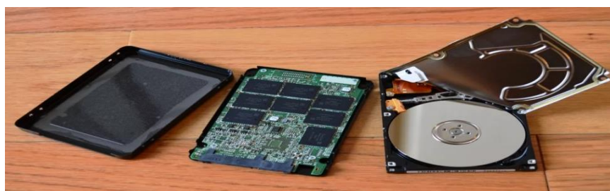
Figure 5. HDD vs. SSD Comparison. Similar outside appearance, however, no common internally of an SSD and HDD (Ngo, 2013)
