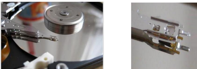
Figure 3. Actuator Arm. Left: The Actuator arm will swing the head back and forth to ensure it is in the exact position on the drive. Right: The extreme tiny end of the hard drive that writes to and reads from the platter (Woodford, 2015)
