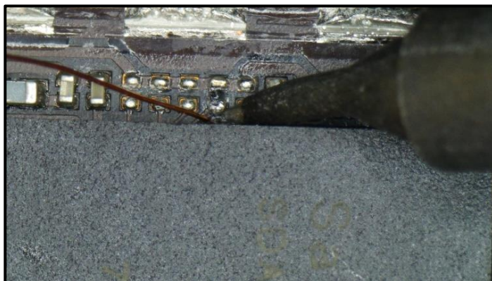
Figure 33 - Soldering to ISP locations to create EDL Mode
