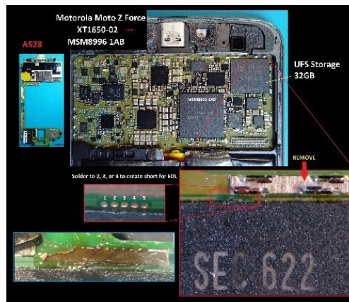
Figure 32 - Motorola XT1650-02 Shorting
