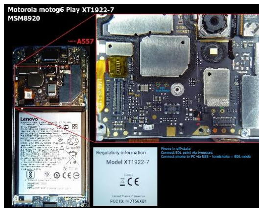
Figure 29 - Motorola motog6 Play XT1922-7 Test Points
