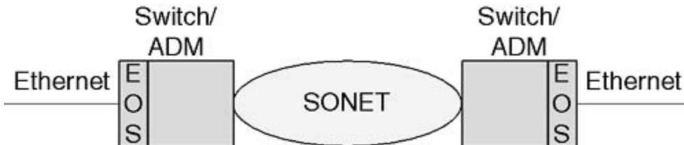
Figure 2-4. EOS and Switching Functions Inside the ADM
