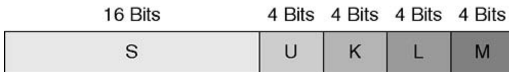
Figure 8-9. SONET/SDH Label Format
