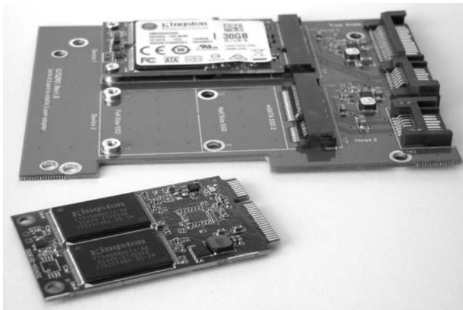
Figure 1-9: mSATA disk interface
