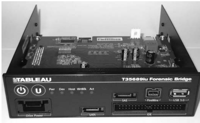
Figure 4-2: Multifunction drive bay write blocker
