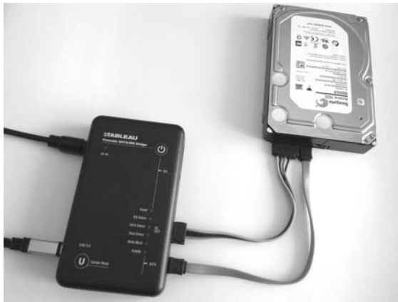
Figure 4-1: Portable SATA write blocker
