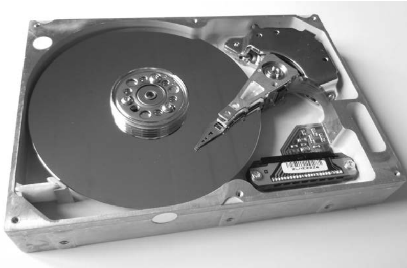
Figure 1-1: Magnetic hard disk
