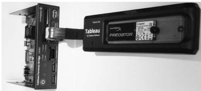
Figure 4-4: Multifunction write blocker and dock for PCI Express M.2 drives
