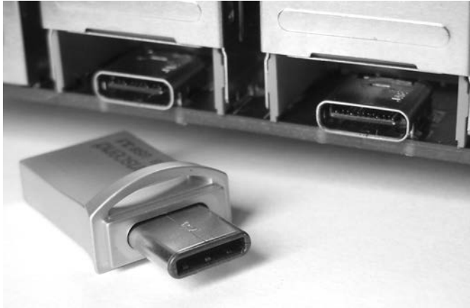
Figure 1-20: USB Type C interface
