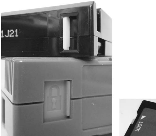
Figure 4-5: Write-protect tabs on tapes and SD cards
