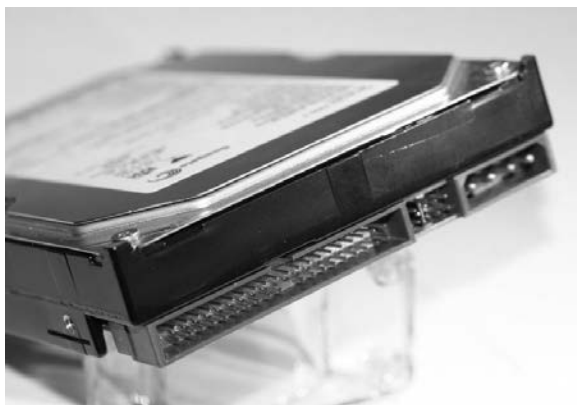
Figure 1-22: IDE disk interface
