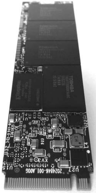
Figure 1-11: M.2 disk interface
