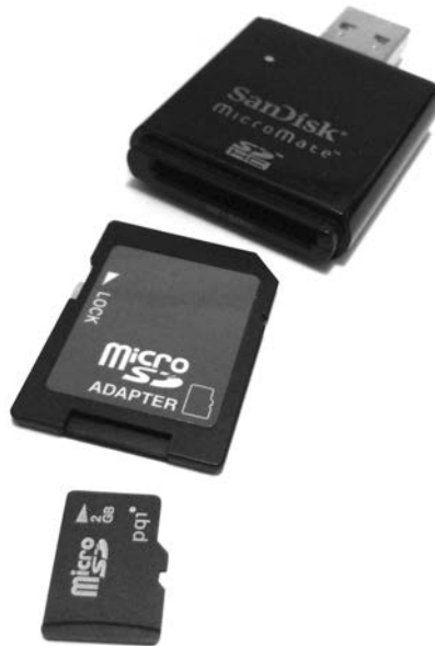
Figure 6-1: Removable memory card adapters
