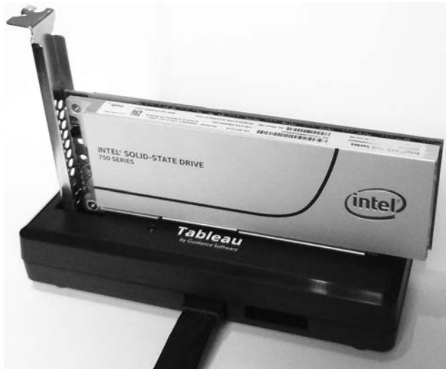
Figure 4-3: Write blocker dock for PCI Express slot drives
