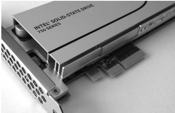
Figure 1-16: NVME SSD with a PCIe interface
