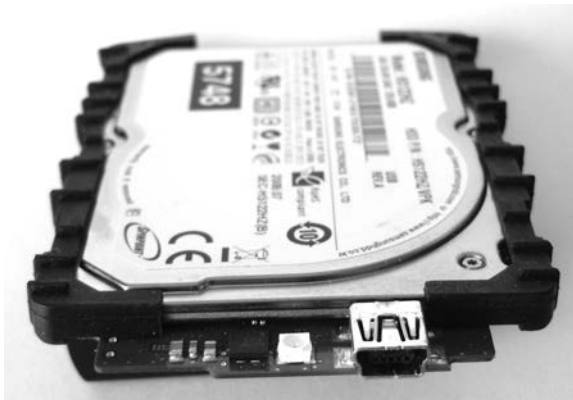
Figure 1-19: A 1.8-inch magnetic hard disk with integrated USB interface
