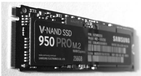
Figure 1-17: NVME SSD with an M.2 interface
