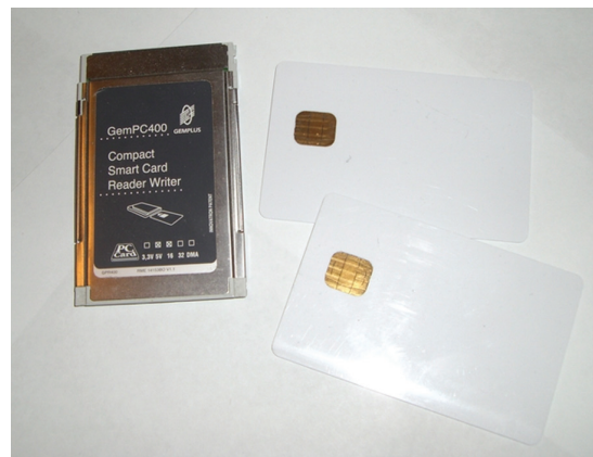
• Figure 8.9 Smart cards have an internal chip as well as multiple external contacts for interfacing with a smart card reader.
