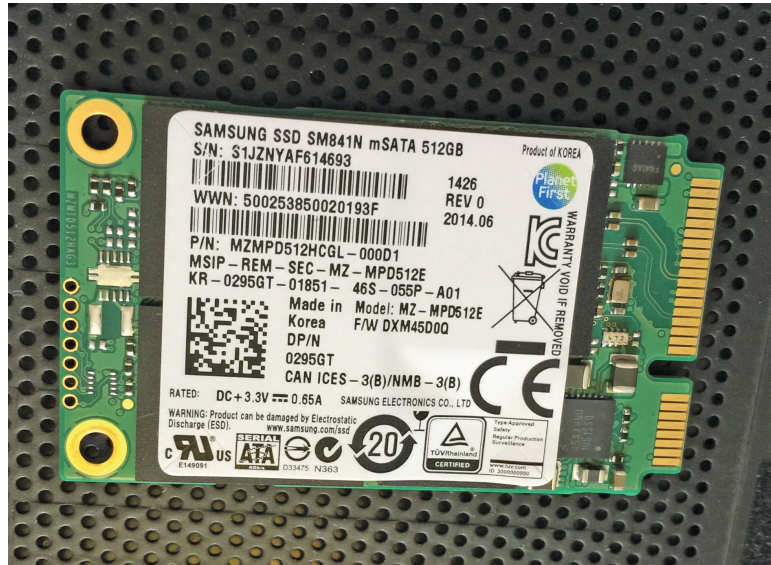
• Figure 10.10 512GB solid state half-height minicard
