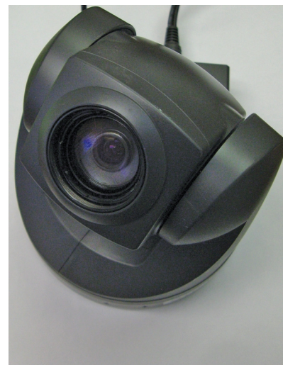
• Figure 8.8 IP-based cameras leverage existing IP networks instead of needing a proprietary CCTV cable.
