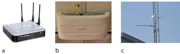
• Figure 12.4 Wireless access point antennas
