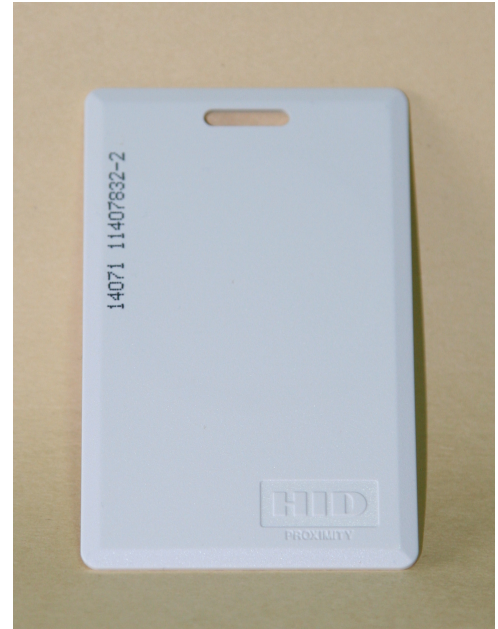
• Figure 8.5 Contactless access cards act as modern keys to a building.
