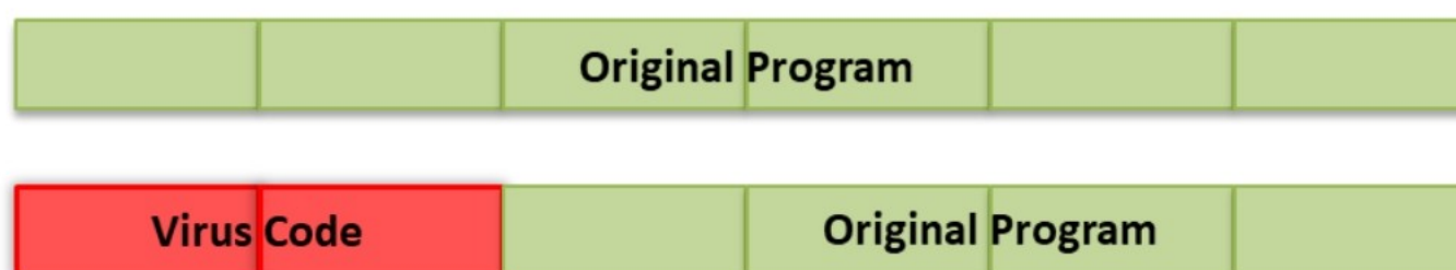
Figure 7.53: Working of intrusive virus
