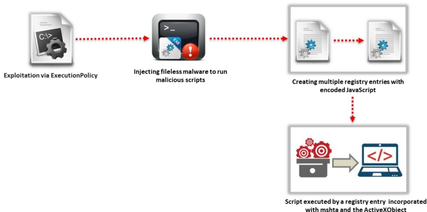
Figure 7.73: Launching fileless malware through Windows registry
