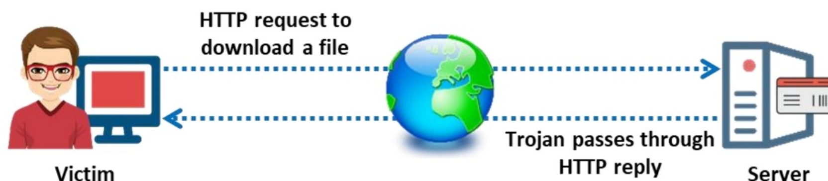
Figure 7.20: Working of HTTP Trojan
