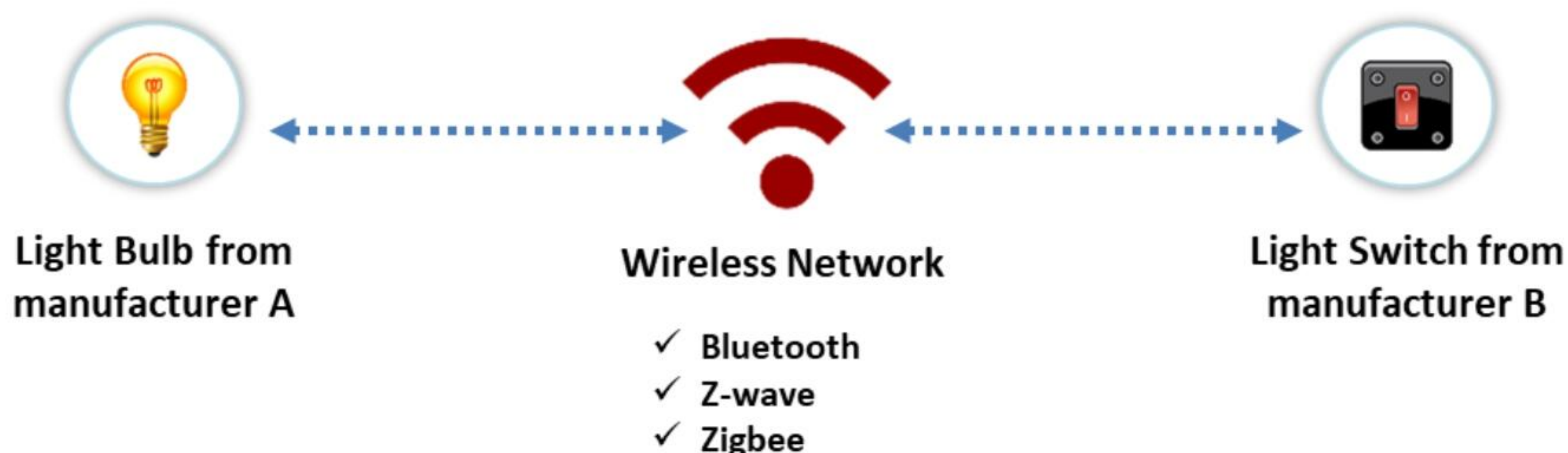
Figure 18.3: IoT device-to-device communication model
