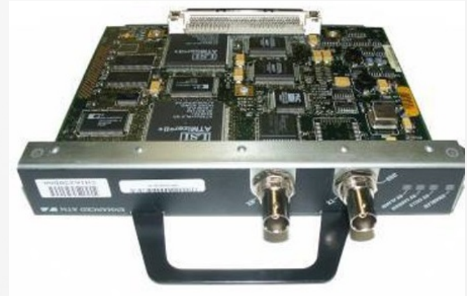
1-Port ATM Enhanced DS3 Port Adapter PA-A3-T3
