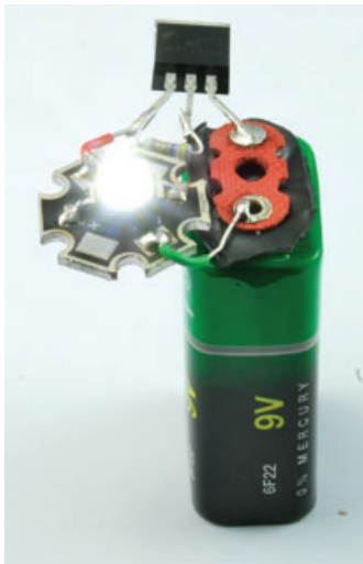
FIGURE 4-13 Emergency LED lighting
