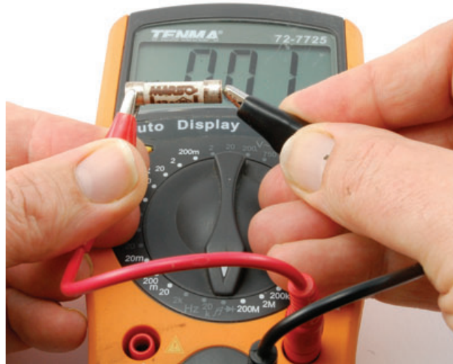
FIGURE 10-3 Testing a fuse with a multimeter
