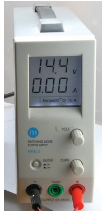
FIGURE 11-7 A lab power supply
