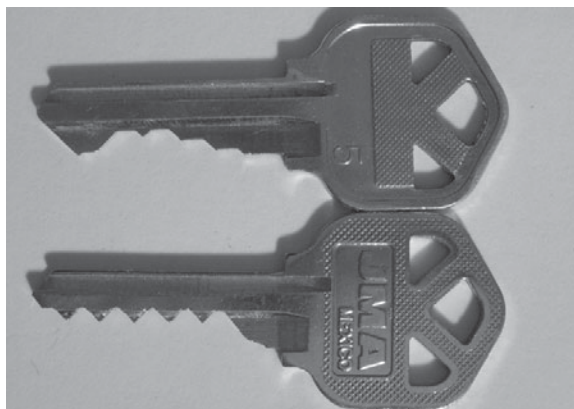
Figure 9-2 A standard key (top) compared to a bump key (bottom). Notice the short, even-height teeth on the bump key.
