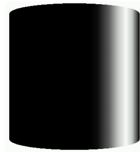
Figure 7–19. A cylinder illuminated with a specular light source
