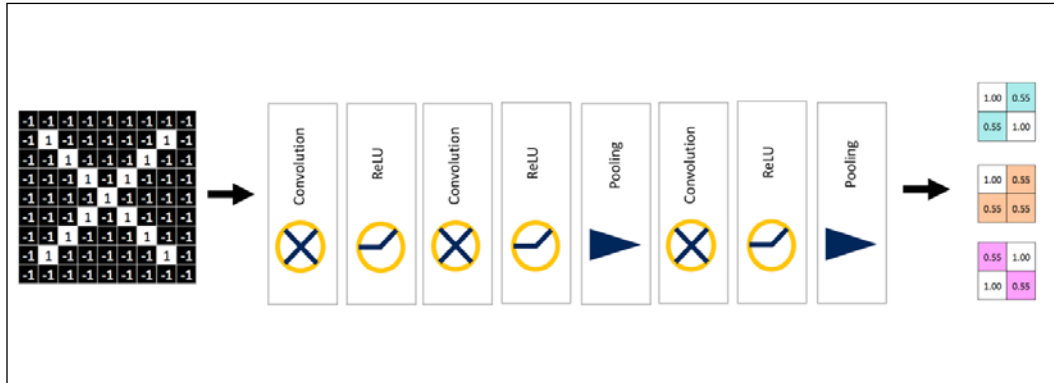
Figure 28: Deep-stacking the basic units repeatedly to form CNN layers.
