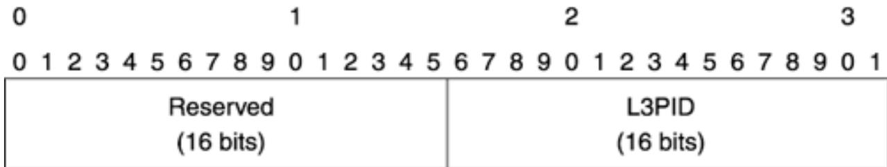
The LABEL\_REQUEST object requests a label. An RSVP\_LABEL object responds to it. The LABEL\_REQUEST object is seen only in Path messages. It contains, in the upper 16 bits, the Layer 3 Protocol Identifier (L3PID) that is carried in the label. Cisco IOS always signals 0x800 (IP); the existence of the L3PID is somewhat historical. The fact that the LABEL\_REQUEST object exists is enough to tell the downstream node that it is expected to provide a label.
