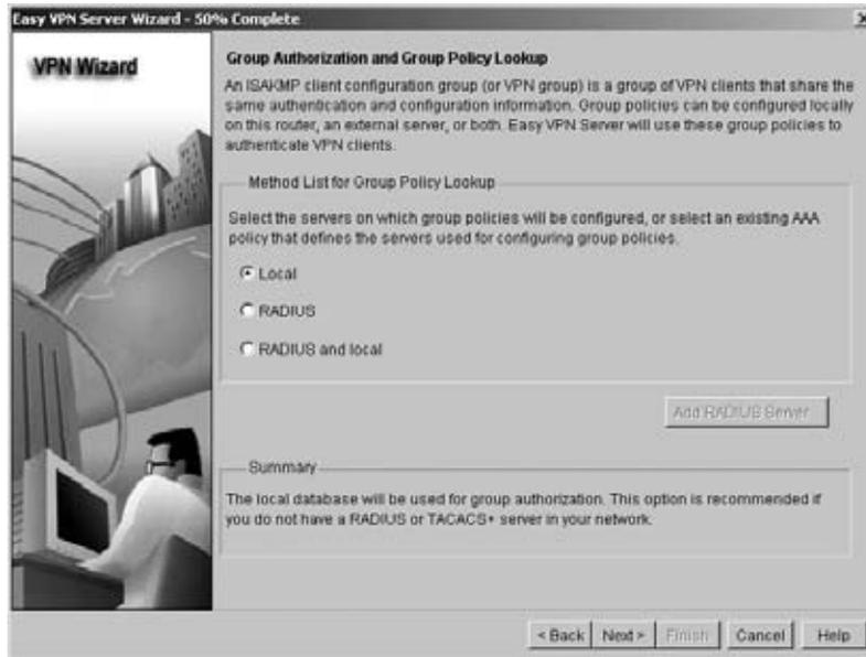
**FIGURE 12.18** Cisco Router and Security Device Manager Create Easy VPN Server XAuth
