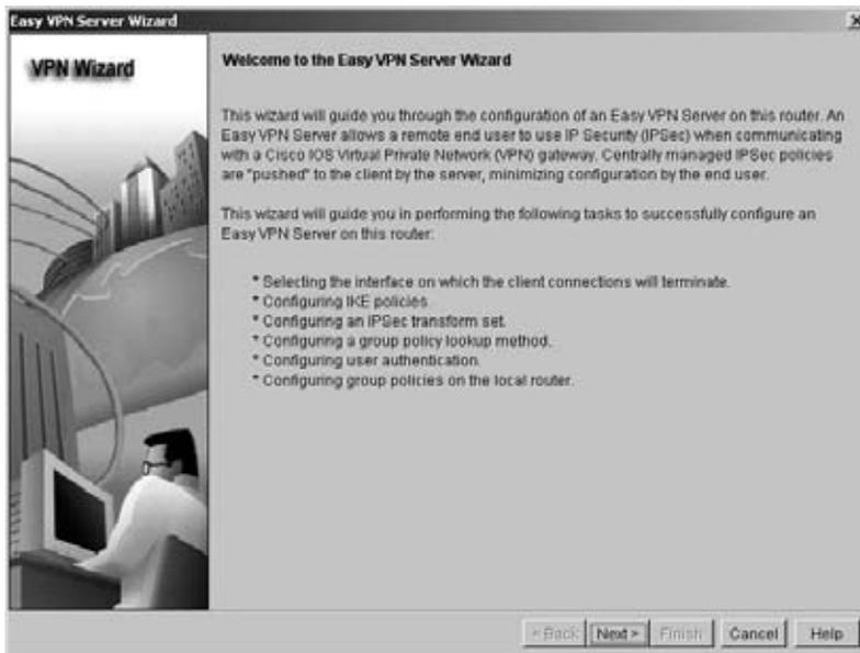
**FIGURE 12.14** Cisco Router and Security Device Manager Create Easy VPN Server Interface and Authentication
